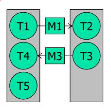
**Step 1**:  $T_1$  (resp  $T_3$ ) has higher priority than successor  $T_2$  (resp  $T_4$ ) Priorities are computed with DMS and  $D_1$  (resp  $D_3$ ) <  $D_2$  (resp  $D_4$ )
